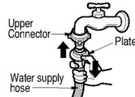
• In case the diameter of the tap is large remove the guide plate.
