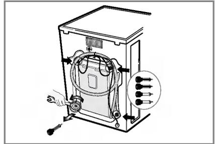
1. To prevent internal damage during transport, the special 4 bolts are locked. Before operating the washer, remove the bolts along with the rubber bungs.
